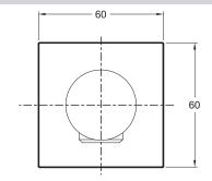
Product Specification: Wall elbow - Square plate. E8467. Collection: MODULO. DIMENSIONS: 13.50 x 9 x 6.50 cm. WEIGHT: 0.5 kg. MATERIAL: Metal. INSTALLATION TYPE: Wall-mount. With non-return valve.
