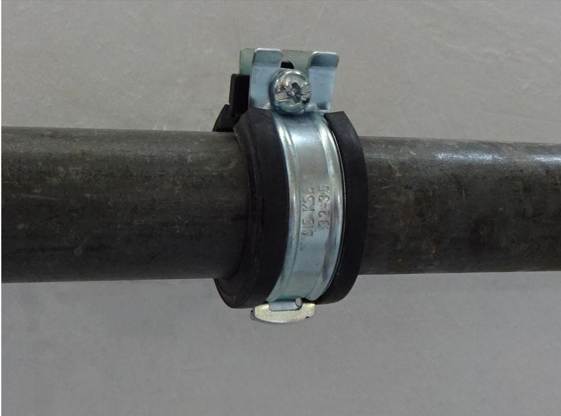
Fig. 2: Meas. 3: KSB1 one-screw-clamp, 2" (59 - 63 mm), connection M8/10, with EPDM-rubber (20 x 4,20 mm)
