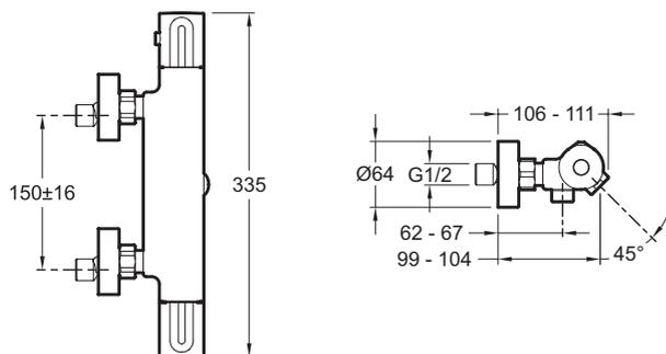
Product Specification: Single-lever thermostatic wall-mount bath/shower mixer. E24395. Collection: MÉTRO. MATERIAL: Metal. INSTALLATION TYPE: 2 holes. TYPE: Single-lever. CONNECTION: With connectors and wall escutcheons. HOLE CONFIGURATION: 150 ± 15. WATER/ENERGY-SAVING: WATER-SAVING. INSTALLATION TYPE: 2 holes. SAFETY STOP: 37°C. MAXIMUM TEMPERATURE: 50°C. WARM BODY: Yes. DIVERTER: Diverter built into handle. MECHANISM GUARANTEE: 5 years. FINISH GUARANTEE: 10 years.
