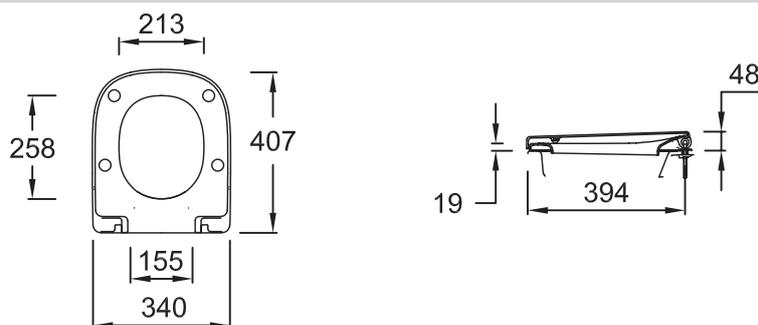
Product Specification: Compact thermoset toilet seat. E4272. Collection: STRUKTURA. WEIGHT: 2.3 kg. MATERIAL: Thermoset. NORMS AND REGULATION: NF.
