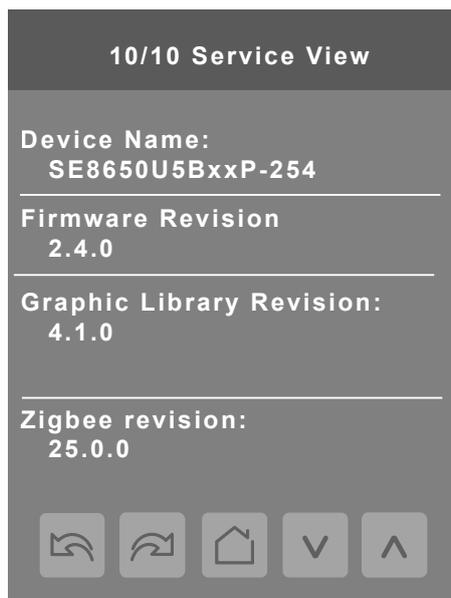
The Device Name (BACnet name) consists of the model number followed by the COM address (MAC address). The BACnet name can be changed via the BACnet front end and the new name appears on the above screen.
