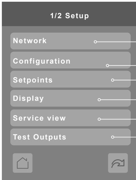
Network — BACnet MS/TP, Modbus, Zigbee and Wi-Fi network settings (Zigbee network settings appear only if Zigbee feature is available)
