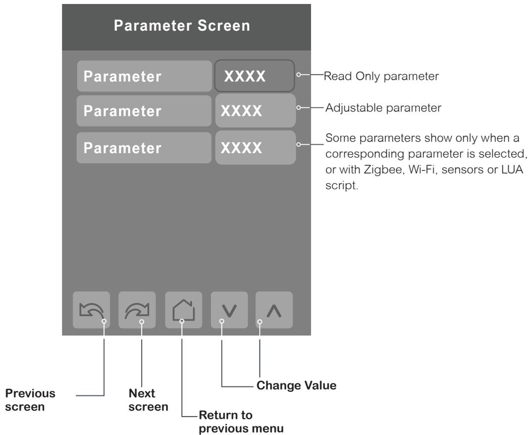
**NOTE:** When any change is made to a parameter, the value is automatically saved in memory when the next parameter is selected or another screen is opened. This event is true only if a parameter was changed locally on the RC. Making changes through BACnet will not have the same outcome. If changes need to be done remotely through BACnet, use priority 1, 2 or 3, or write to relinquish default (priority 17).
