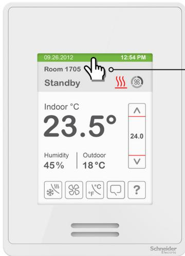
Touch and hold this point for 3 seconds to enter setup mode
