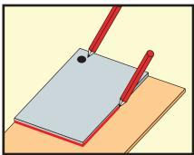
**Step 2)** using a single sheet of marine plywood with a minimum thickness of 12mm mark the trays perimeter and waste hole. Fit all waste services before securing your plywood to your joists. (For sizing please refer to **Fig A** on opposite page)
