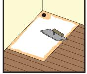
Manipulate tray a minimum of 5mm into bed to ensure the underside of the tray is fully supported.
