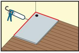
**Step 6)** Run a further bead of neutral mould resistant silicone around the rims of the tray adjacent to all walls. Allow all aspects of material to cure according to the manufacturers instructions.
