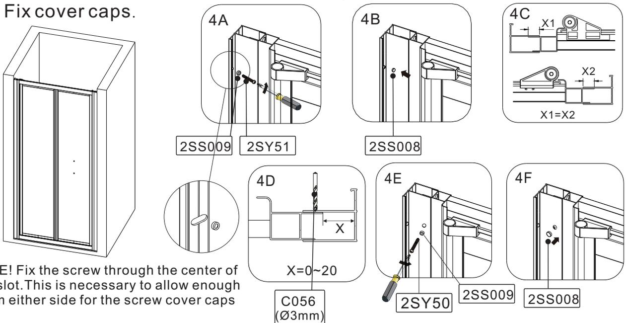
NOTE! Fix the screw through the center of the slot. This is necessary to allow enough room either side for the screw cover caps
