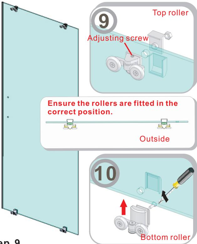
Ensure the rollers are fitted in the correct position.
