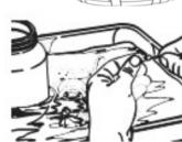
9. Clean the container, suction tube, air cap and nozzle with a cleaning brush and the appropriate cleaning solution.
