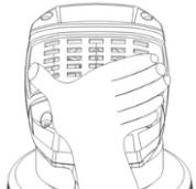
2. Remove the dirty filters and replace with new ones.
