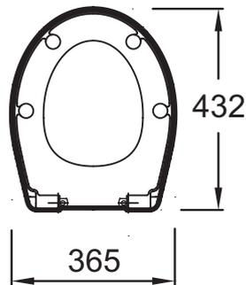
Product Specification: Polypropylene toilet seat. E4357G. Collection: BRIVE. DIMENSIONS: 43.20 x 36.50 cm. WEIGHT: 1.2 kg. MATERIAL: Polypropylene. SEAT TYPE: Standard. HINGES: Adjustable metal.
