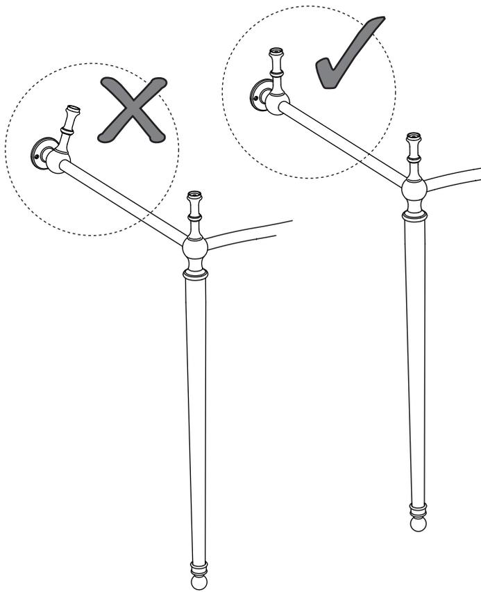
**7** Determine the final installation position and mark the 4 wall and two floor fixing hole positions in pencil. Please make sure to include the floor nipples (and washers if necessary) when determine the installation position because the stand may elevate after the floor nipples are fitted.
