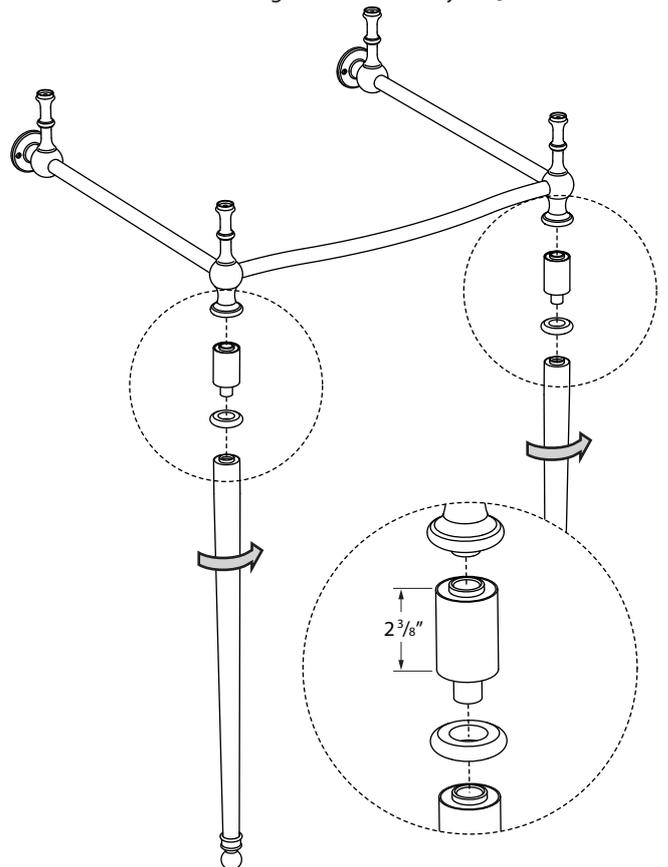
**6** Check that the horizontal bracket bar is vertical using a spirit level.
