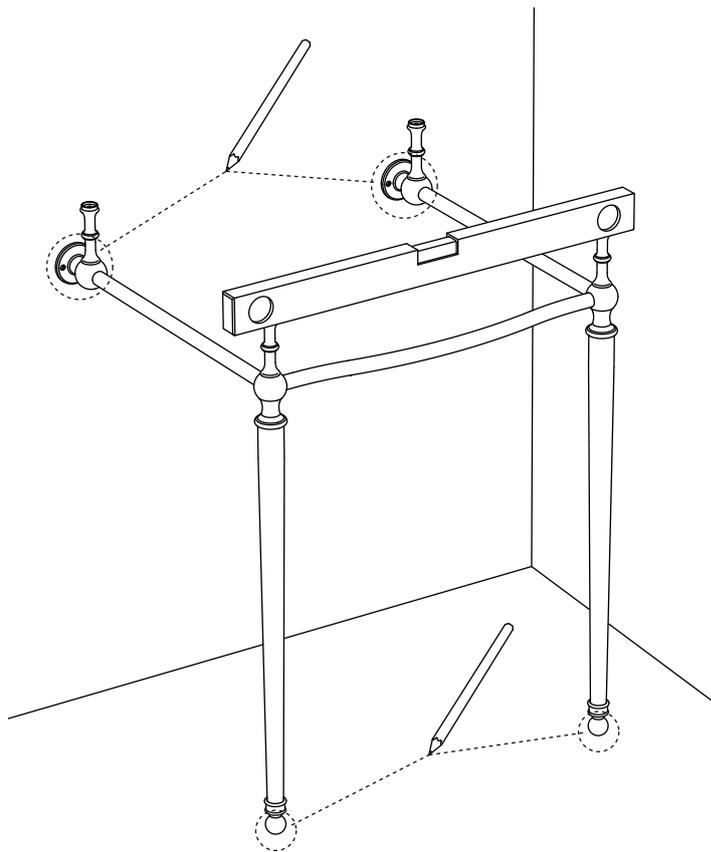
**8** Using a 1/4" drill bit drill the six holes on the marked positions. **Note:** In the event that the wall / floor fixings supplied being inappropriate for the wall / floor, please source alternatives.
