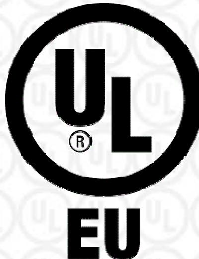
The minimum height of the registered trademark symbol ® shall be 1 mm. When the overall diameter of the UL-EU Mark is less than 9.5 mm, the trademark symbol may be omitted if it is not legible to the naked eye.
