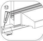
**Note:** Remove spacers in frame. Insert seal **8SSJ074** into the top and bottom profile. On both ends, pull out 30mm and put silicone on the top of the seal and reinsert.
