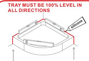
Ensure the shower tray is level in all directions and is properly sealed to the wall. The wall must be tiled down to the top edge of the tray. **Do not angle out bottom tile**.
