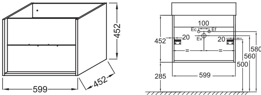
Product Specification: Base unit for vanity top 60 cm, 2 drawers, no handles. EB1583-N18. Collection: VIVIENNE. DIMENSIONS: 59.90 x 45.20 x 45.20 cm. WEIGHT: 23 kg. MATERIAL: Lacquer and melamine. INSTALLATION TYPE: Wall-hung. LIGHTING: No. USB SOCKET: No. HANDLE : 0. INSIDE FINISH: Grey. FIXING: Installer selects fixings set according to wall support.
