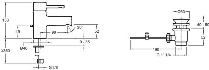
Product Specification: Single-lever washbasin mixer. E37301. Collection: CUFF. WEIGHT: 1.3 kg. MATERIAL: 54. INSTALLATION TYPE: 1 hole. NORMS AND REGULATION: ACS (Certificate of Sanitary Compliance): 10 ACC LY 004. TYPE: Single-lever. FLOW RATE: 5 l/min. HEIGHT UNDER SPOUT: 133. MECHANISM: Ceramic disc cartridge. MECHANISM GUARANTEE: 5 years. Side lift rod. Waste.
