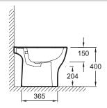
Product Specification: Bidet. EBC0001. Collection: STRUKTURA. DIMENSIONS: 54 x 34 cm. WEIGHT: 18.9 kg. MATERIAL: Ceramic. INSTALLATION TYPE: Floor-standing. HEIGHT: Standard. PRODUCT INCLUDED: (Tap not included). TOILET BOWL FIXINGS: Concealed.
