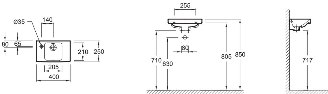
Product Specification: Handwash basin 40 cm. E4759G. Collection: ODÉON UP. DIMENSIONS: 40 x 25 cm. WEIGHT: 5.5 kg. MATERIAL: Ceramic. INSTALLATION TYPE: Self-supporting. TAP DRILLING: 1 tap hole. INSTALLATION: COMPACT. OVERFLOW: With overflow hole. RECOMMENDED TAPS: Aleo, a stylish, affordable range.
