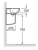
Product Specification: Handwash basin 45 cm. E4760. Collection: ODÉON UP. DIMENSIONS: 45 x 32 cm. WEIGHT: 8.5 kg. MATERIAL: Ceramic. INSTALLATION TYPE: Self-supporting or can be mounted on a specific cabinet. FAUCET DRILLING: 1 tap hole. TAP DRILLING: 1 tap hole. INSTALLATION: STANDARD. OVERFLOW: With overflow hole. PRODUCT INCLUDED: (Tap not included). RECOMMENDED TAPS: Aleo, a stylish, affordable range.
