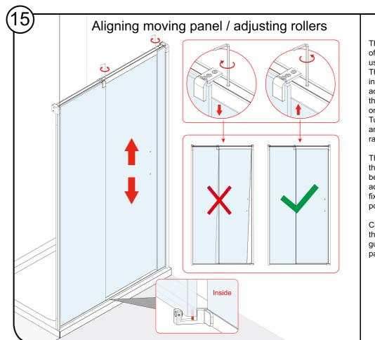
The height and alignment of the door can be adjusted using the hex key provided. The moving panel must be in the closed position to access the adjusting screw through the access ports on the top of the rail. Turn clockwise to lower and anti-clockwise to raise.
