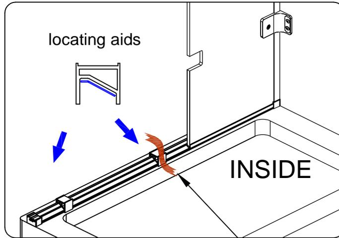
Tip! Hold both locating aids in position with masking tape.
