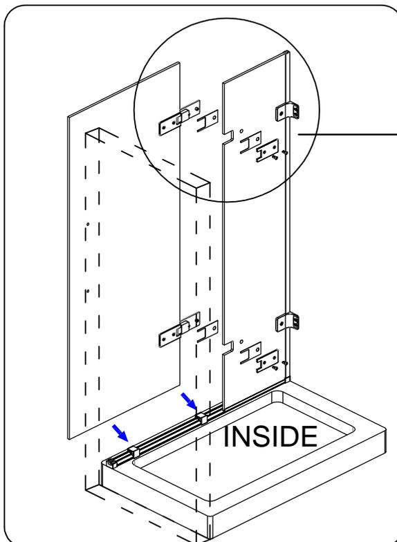
Use door assembly tool to hold the door in place until the hinges are fitted.
