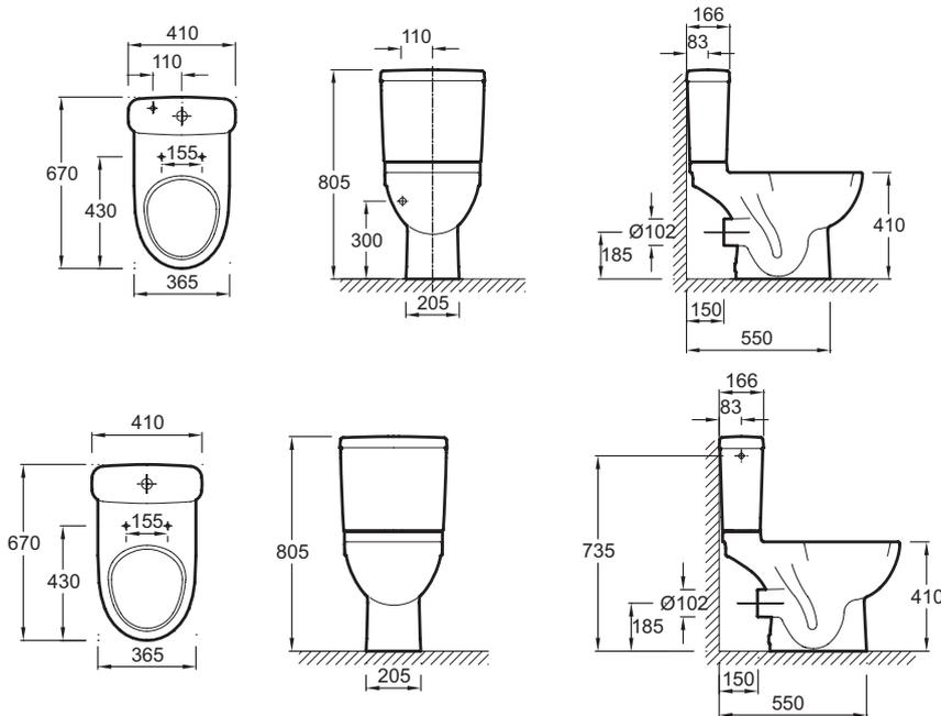
Product Specification: WC pan, P-trap. 4956CK. Collection: ODÉON UP. DIMENSIONS: 67 x 36.50 cm. WEIGHT: 23.5 kg. MATERIAL: Ceramic. INSTALLATION TYPE: Floor-standing. VOLUME OF WATER: 2.6/4 L and 3/6 L. HEIGHT: Comfort. RIM TYPE: Open (traditional). RIM: With rim. PRODUCT INCLUDED: (Cistern and seat not included). WATER USE: Water-efficient 2.6/4 L dual flush or 3/6 L standard flush. P-trap. Cistern not included.
