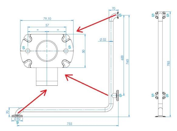
It is recommended to install the grab bar between 700 and 750 mm high from floor.
