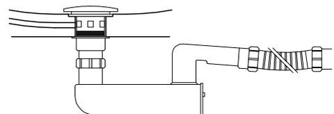
dettaglio piletta / close-up view of waste kit
