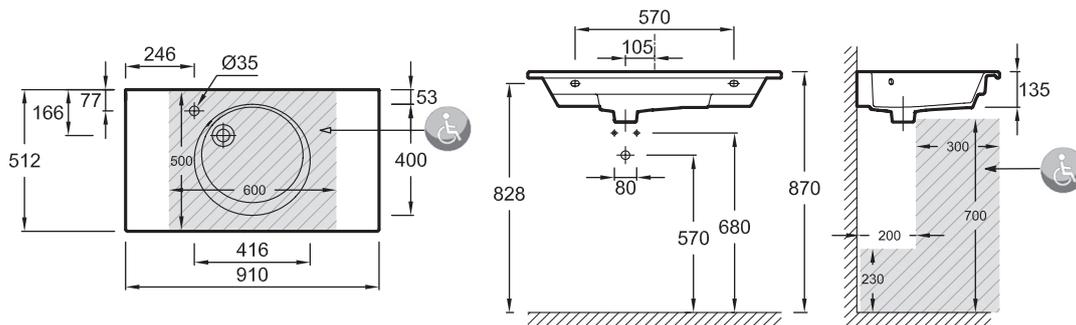
Product Specification: Vanity top 90 cm. EXAV112. Collection: ODÉON RIVE GAUCHE. DIMENSIONS: 91 x 51.20 cm. WEIGHT: 23.2 kg. MATERIAL: Ceramic. INSTALLATION TYPE: Self-supporting. TAP DRILLING: 1 tap hole. OVERFLOW: With. RECOMMENDED BRASSWARE: Odéon Rive Gauche (several finish options).
