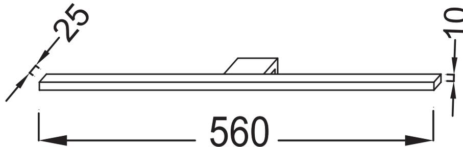
Product Specification: "Eclat" LED spotlight. EB1237. Collection: NO COLLECTION. DIMENSIONS: 56 x 2.50 x 1 cm. WEIGHT: 0.4 kg. MATERIAL: Metal. INSTALLATION TYPE: Wall-mount. POWER: 230V, 7W, Class II IP44. TEMPERATURE: 4000°K.
