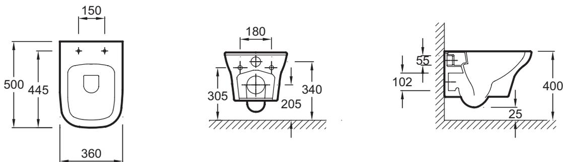
Product Specification: Rimless wall-hung WC Pack. EDM112. Collection: VOX. DIMENSIONS: 50 x 36 cm. WEIGHT: 25 kg. MATERIAL: Ceramic. INSTALLATION TYPE: Wall-hung. VOLUME OF WATER: Standard 3/6 L. HEIGHT: Comfort. RIM TYPE: Rimless. SEAT TYPE: Extra-slim, removable, slow-close. PRODUCT INCLUDED: (seat included). TOILET BOWL FIXINGS: Invisible.
