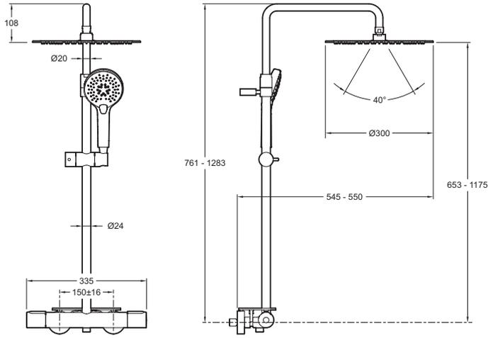
Product Specification: Shower column. E26588. Collection: MÉTRO. DIMENSIONS: 33.40 x 54.60 x 131.50 cm. WEIGHT: 5.6 kg. MATERIAL: Metal. INSTALLATION TYPE: Wall-mount. SHOWER TAPS-WATER/ENERGY SAVING: Water-saving. WITH OR WITHOUT BRASSWARE: WITH FITTINGS. SINGLE-LEVER TAPS: Thermostatic. SHOWER TAPS-DIVERTER: Integrated. SHOWER TAPS- SAFETY STOP: 37°C. SHOWER TAPS-MAXIMUM TEMPERATURE: 50°C. SHOWER TAPS-HANDSHOWER FLOW: 10 L/min. HOSE TYPE: Smooth, anti-twist, metal look. NUMBER OF SPRAYS: 3.
