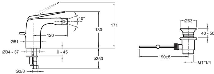
Product Specification: Single-lever bidet mixer with supply hoses. E97014. Collection: AVID. WEIGHT: 1.4 kg. MATERIAL: Brass. INSTALLATION TYPE: 1 hole. TYPE: Single-lever. FLOW RATE: 5 l/min. CONNECTION: With supply hoses. WASTE : With waste. INSTALLATION TYPE: 1 hole. MECHANISM GUARANTEE: 5 years. Rotating anti-scale aerator. Metal cartridge pin.
