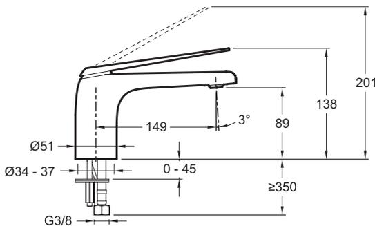
Product Specification: Single-lever monobloc basin mixer - with supply hoses. E97345-ND. Collection: AVID. WEIGHT: 2.2 kg. MATERIAL: Brass. INSTALLATION TYPE: 1 hole. TYPE: Single-lever. FLOW RATE: 5 l/mn. HEIGHT UNDER SPOUT: 138. SPOUT PROJECTION: 149. CONNECTION: With supply hoses. MECHANISM: Ceramic disc cartridge. WASTE : Without waste. INSTALLATION TYPE: 1 hole. MECHANISM GUARANTEE: 5 years. Metal cartridge pin. Height under aerator: 89 mm. No lift rod or waste.
