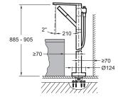
Product Specification: Shower-bath mixer with underfloor supply. E73087. Collection: COMPOSED. WEIGHT: 12 kg. MATERIAL: Brass. INSTALLATION TYPE: Floor-mount. TYPE: Single-lever. MECHANISM: Ceramic disc cartridge. WASTE: Without waste. INSTALLATION TYPE: 1 hole. DIVERTER: Automatic diverter at rear of spout. MECHANISM GUARANTEE: 5 years. HOSE TYPE: Smooth, anti-twist hose. Install with floor base 97906D.
