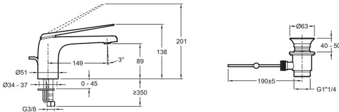
Product Specification: Single-lever wall-mount washbasin mixer with supply hoses. E97345. Collection: AVID. WEIGHT: 2.2 kg. MATERIAL: Brass. INSTALLATION TYPE: 1 hole. TYPE: Single-lever. FLOW RATE: 5 l/min. CONNECTION: With supply hoses. MECHANISM: Ceramic disc cartridge.. INSTALLATION TYPE: 1 hole. MECHANISM GUARANTEE: 5 years. Height under aerator: 89 mm. Spout reach: 149 mm. Metal cartridge pin.
