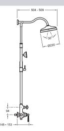
Product Specification: Shower column. E24311. Collection: CLÉO 1889. DIMENSIONS: 133 x 26 x 14.80 cm. WEIGHT: 5.4 kg. MATERIAL: Metal. INSTALLATION TYPE: Wall-mount. SHOWER TAPS-WATER/EN-ERGY SAVING: Water-saving. WITH OR WITHOUT BRASSWARE: WITH FITTINGS. SHOWER TAPS-HANDSHOWER FLOW: 9 L/min. NUMBER OF SPRAYS: 5.
