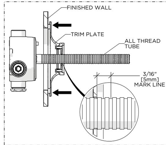
2. Firmly holding the PLATE against the finished wall, mark the TUBE 3/16" [5mm] beyond where it protrude from the PLATE.
