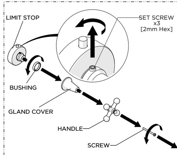
11. Unthread the SCREW, remove the HANDLE, remove the GLAND COVER, and unthread the BUSHING to expose the SET SCREWS then loosen the SET SCREWS using a 2mm hex key.
