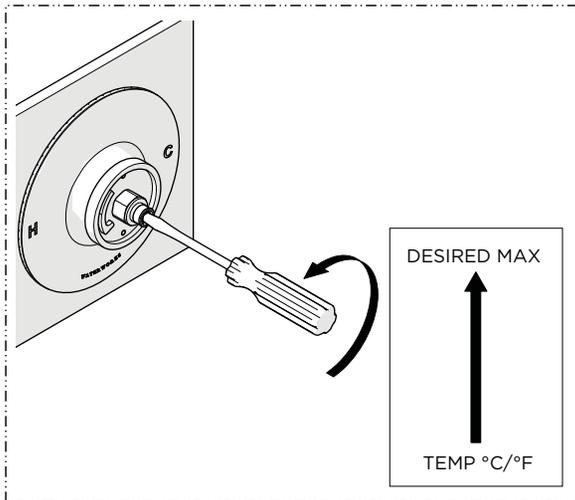
10. With water running, rotate the SQUARE TUBE to adjust the temperature to the maximum desired bathing temperature, verified with a thermometer. Turn the water off and make sure not to change this setting.
