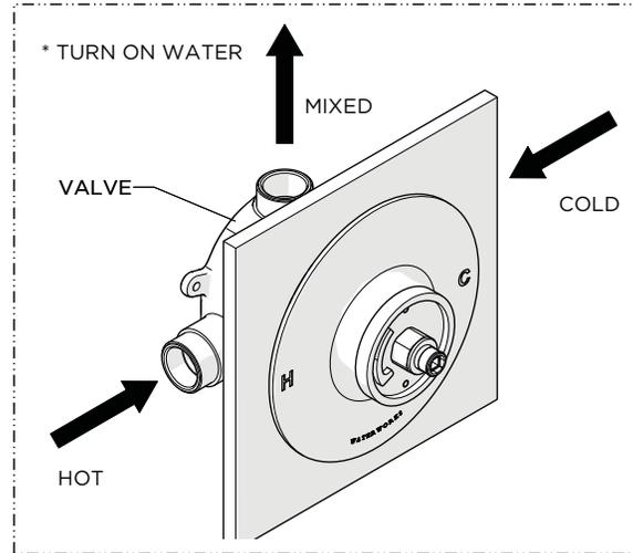
8. Turn on the water supply and open a diverter or wall valve (sold separately) to run water through the thermostatic valve.
