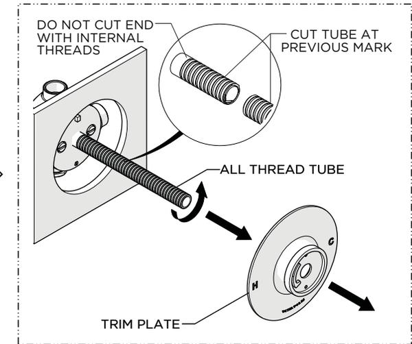
3. Remove the TRIM PLATE and ALL THREAD TUBE, then cut the TUBE at the previous mark. Do NOT cut the end with the internal threads.
