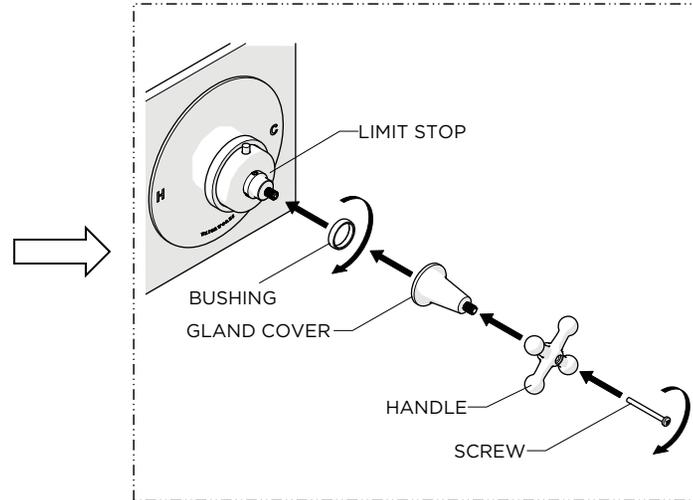
14. Thread the BUSHING back onto the LIMIT STOP, place the GLAND COVER onto the LIMIT STOP and over the BUSHING, place the HANDLE onto the GLAND COVER in the desired orientation, then thread and securely tighten the SCREW.
