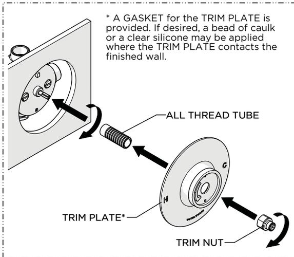
4. Thread the TUBE back onto the CARTRIDGE, slide the PLATE over the TUBE, and thread the TRIM NUT onto the TUBE. Securely tighten to hold the PLATE against the finished wall.
