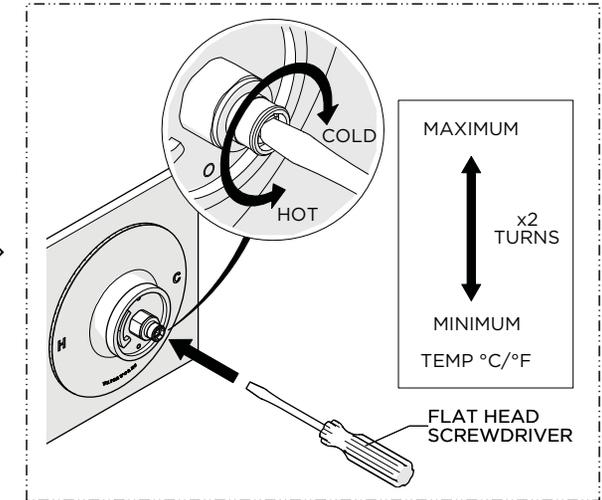
9. Insert a bladed screw driver into the SQUARE TUBE. Slowly rotate the TUBE clockwise to attain full cold then counterclockwise to attain full hot. It's approximately 2 complete rotations. Verify a full range of temperatures exists.
