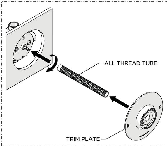
1. Thread the ALL THREAD TUBE onto the CARTRIDGE then slide the TRIM PLATE over the TUBE.
