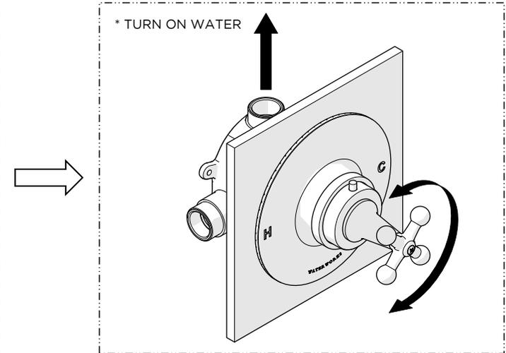
15. Turn on the water supply and operate the HANDLE to ensure that it is functioning properly.
