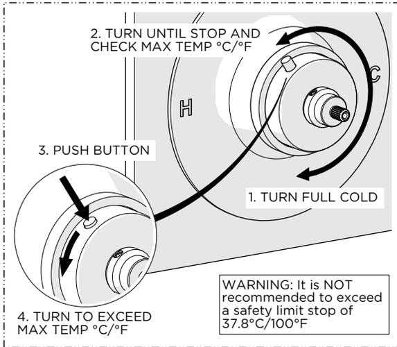
13. Turn the LIMIT STOP to cold then hot and confirm it is functioning properly. Verify the maximum desired bathing temperature. To get a hotter temperature, press and hold the LIMIT STOP BUTTON and turn the LIMIT STOP further.
