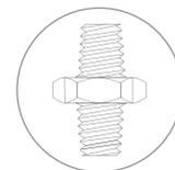
\*\* NPT tapered (conical) ANSI/ASME B1.20.1
